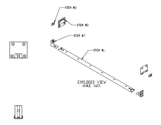
In order to have access to the screws thru the stiffener into the bottom shelf of the cabinet, build from the top down.
